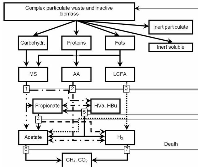
**Figure 1.** The anaerobic model as implemented including biochemical processes: (1) acidogenesis from sugars, (2) acidogenesis from amino acids, (3) acetogenesis from LCFA, (4) acetogenesis from propionate, (5) acetogenesis from butyrate and valerate, (6) aceticlastic methanogenesis, and (7) hydrogenotrophic methanogenesis (Batstone *et al.*, 2002b)
