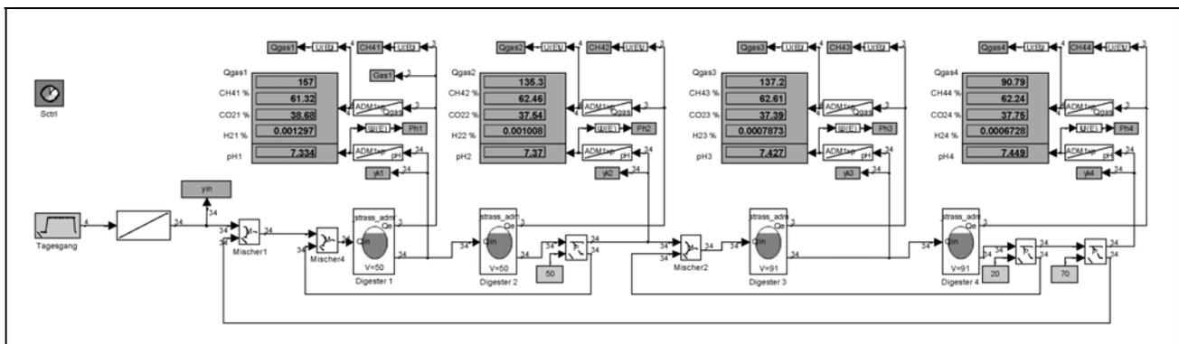
**Figure 5.** 4-chamber system represented by serial ADM1 digesters edited in the SIMBA-environment for the simulation of gas production in individual chambers
