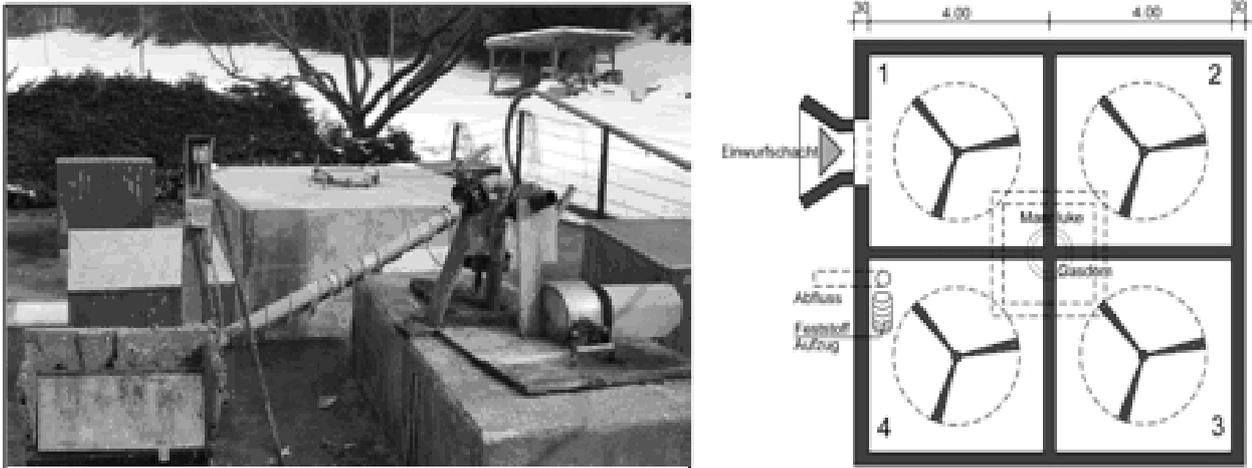
**Figure 2.** 4-chamber biogas plant for co-fermentation of piggery manure and biowaste with a total volume of 190 m<sup>3</sup>
