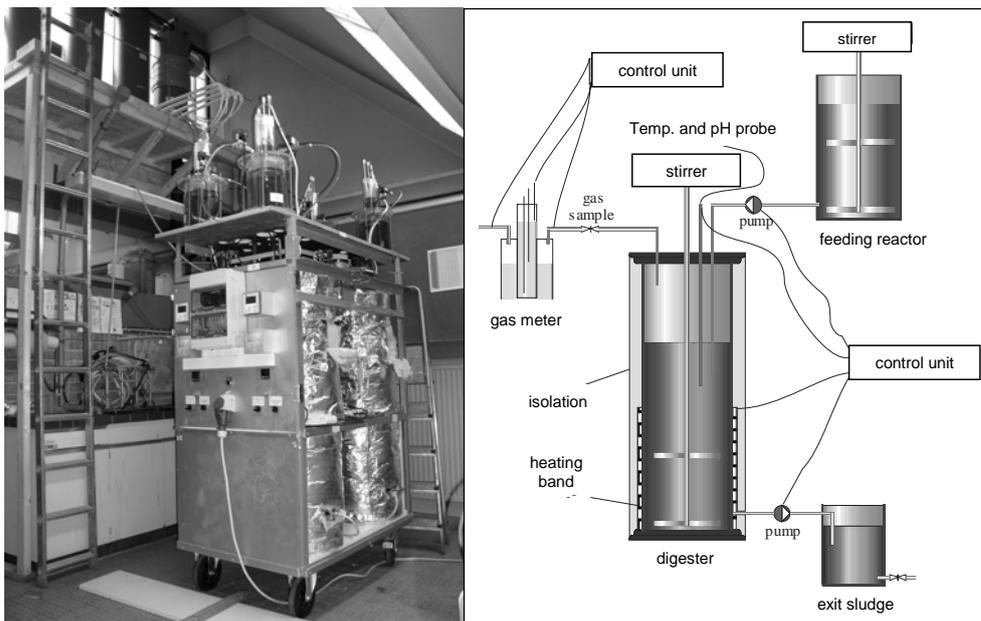
**Figure 3.** Set-up of 4 lab-scale digesters with a volume of 0.1 m<sup>3</sup> each for parallel digestion tests
