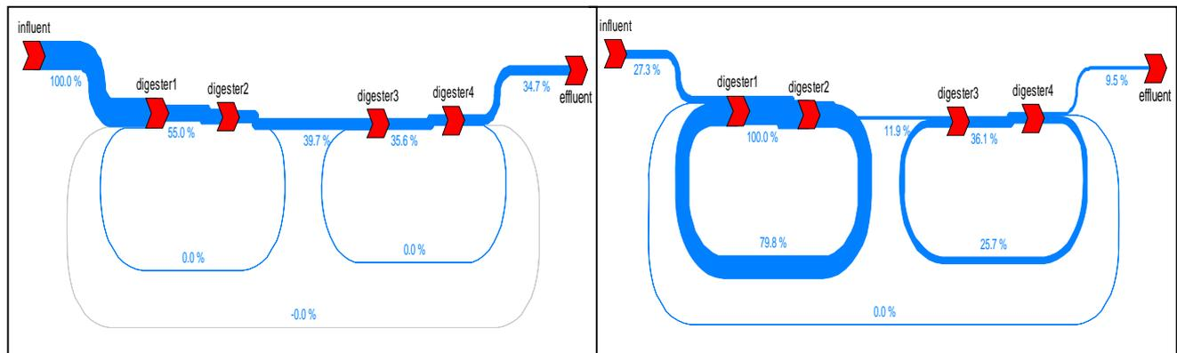
**Figure 8.** Calculated COD degradation for high loading with recycle pumping rates of 0/0 (left) and 50/20 (right), the value for 100 % is related to the largest COD stream including the recycle flux in each case
