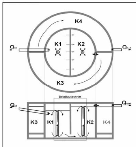
**Figure 4.** Improved flow scheme of the 4-chamber pilot plant with cylindrical shape
