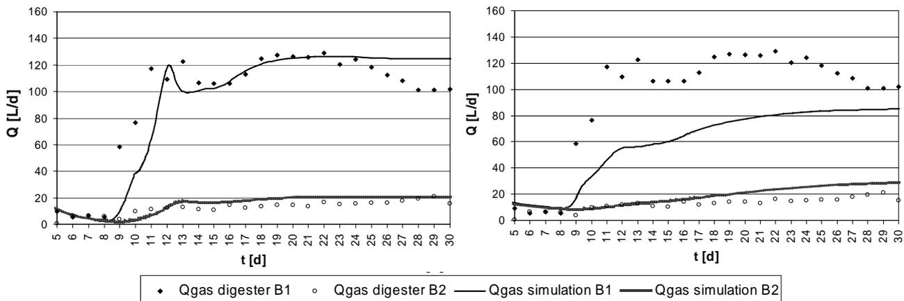
**Figure 6.** Calibration runs for gas production comparing best fit disintegration rate ( $k_{dis} = 0.5$ , left) and default parameter ( $k_{dis} = 0.096$ , right)
