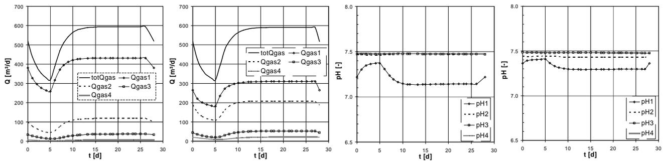
**Figure 7.** Simulated distribution of gas production and pH within the 4 chamber system at high loading with and without recycling (recycle pumping rates of 0/0 and 50/20 from left to right)
